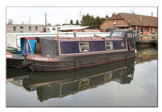
Exterior: Black bitumen painted hull to rubbing band. Black from rubbing band
