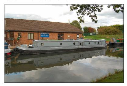
Exterior: Black bitumen painted hull to rubbing band. Light grey from rubbing
