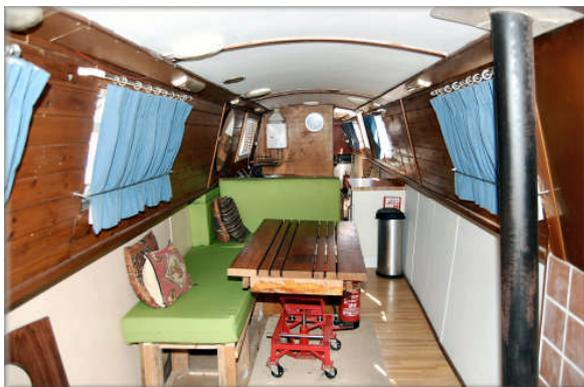
*Cabin 4:* Saloon. At the aft end of the saloon is a fitted L shape seating unit with upholstered foam cushions and dining table. Storage below. This can convert to a double berth. The Hamlet solid fuel stove is mounted on a stone timber trimmed hearth with quarry tiled rear. At the forward end of the cabin a gunnel height angled cupboard. Small step through to forward well that has been converted into storage area.
