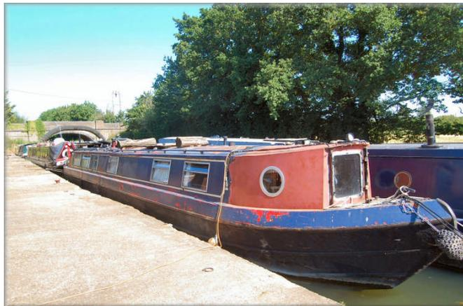
*Exterior:*    Black bitumen painted hull to rubbing band. Dark blue from rubbing band through side decks, cabin sides and roof. Cream coachlines on cabin sides.
