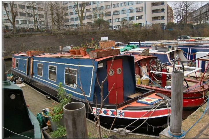
*Exterior:* Black bitumen painted hull to rubbing band. Black from rubbing band through side decks, with non slip finish to side decks. Blue cabin sides with cream coach line, red panels at the stern with name sign written. Red roof.
